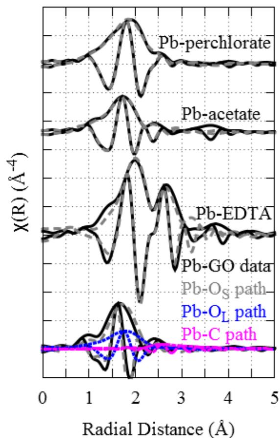
Fig. S.8: FT spectra of Pb(II) aqueous standard compounds showing both the magnitude (all positive) and real part of the data (solid black line) and the best fit line (dashed gray line).
