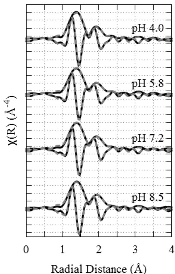
Fig. S.7: FT spectra of the U-MLGO samples at pH 4.0, 5.8, 7.2 and 8.5 with split equatorial oxygen shell showing both the magnitude (all positive) and real part of the data (solid black line) and the best fit line (dashed gray line), [GO] = 0.42 g/L, [U] = 0.010 g/L, [NaClO<sub>4</sub>] = 0.10 M, T = 293 K.
