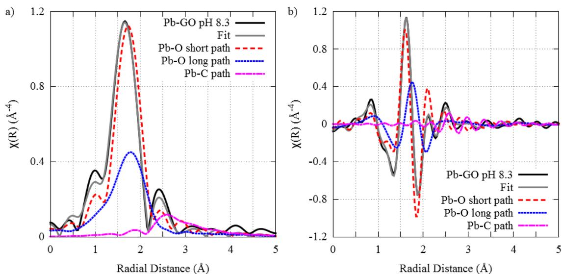
Fig. S.9: FT spectra and paths for the Pb-MLGO pH 8.3 data (black line) in both a) magnitude and b) real part with the fitting paths of the Pb-Os path (dashed red line), the Pb-O<sub>L</sub> path (dotted blue line) and the Pb-C path (dash-dot purple line) combining to form the total fit (gray line).
