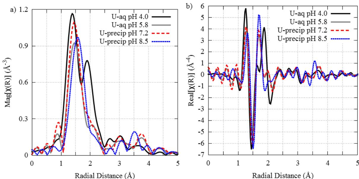
Fig. S.6: EXAFS data for U standards created at pH 4.0, 5.8, 7.2 and 8.5 showing a) the magnitude and b) the real part of the data,  $[\text{U}] = 0.010 \text{ g/L}$ ,  $[\text{NaClO}_4] = 0.10 \text{ M}$ ,  $T = 293 \text{ K}$ .
