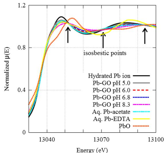
Fig. S.10: Comparison of Pb-MLGO sample data at pH 5.0, 6.0, 6.8 and 8.3 with the Pb aqueous standards and solid PbO in energy space for the near edge (XANES) region, with arrows indicating the isosbestic points, [GO] = 0.42 g/L, [Pb] = 0.010 g/L, [NaClO<sub>4</sub>] = 0.10 M, T = 293 K.
