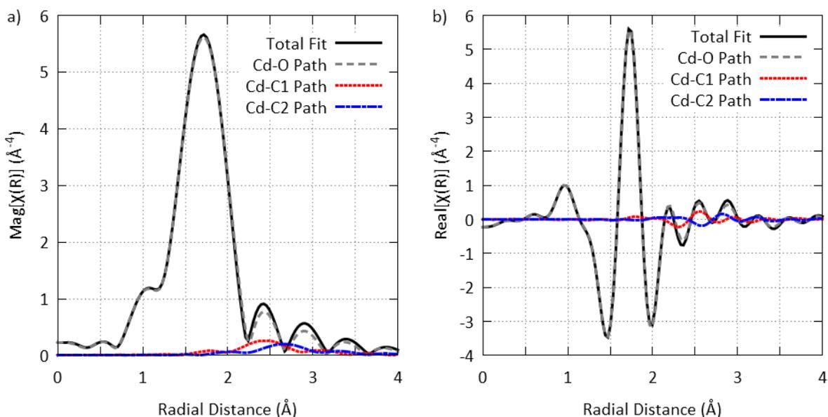
Fig. S.3: Contributing Cd-O (dashed gray line) and two Cd-C paths (dotted red line and dash-dot blue line) demonstrating possible destructive interference from multiple adsorption sites or a floppy monodentate inner sphere bond for a) the magnitude of the FT data (black line) and b) the real part of the FT data (black line). Note the strong similarities between the total fit and the Cd-O path, with the two Cd-C paths contributing almost nothing to the total fit across the fitting range.
