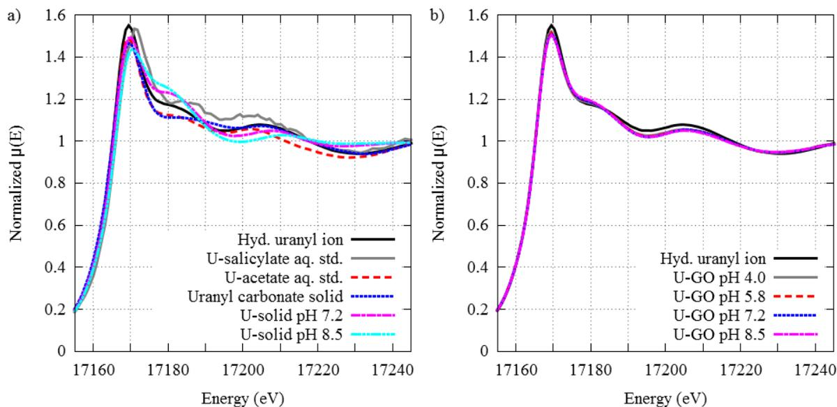
Fig. S.5: XANES data for U-MLGO data showing a) the solid and aqueous standards only and b) just the U-MLGO data at pH 4.0, 5.8, 7.2 and 8.5 with the  $\text{UO}_2^{+2}$  hydrated ion for comparison,  $[\text{GO}] = 0.42 \text{ g/L}$ ,  $[\text{U}] = 0.010 \text{ g/L}$ ,  $[\text{NaClO}_4] = 0.10 \text{ M}$ ,  $T = 293 \text{ K}$ .
