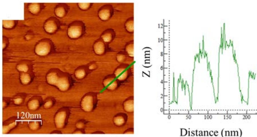
Fig. S.1: AFM image and height profile for the indicated cross-section in green for MLGO particles. Reprinted from Colloids and Surfaces A, 466, T.A. Duster, et al., “Surface complexation modeling of proton and metal sorption onto graphene oxide,” 28-39, 2015, with permission from Elsevier [2].
