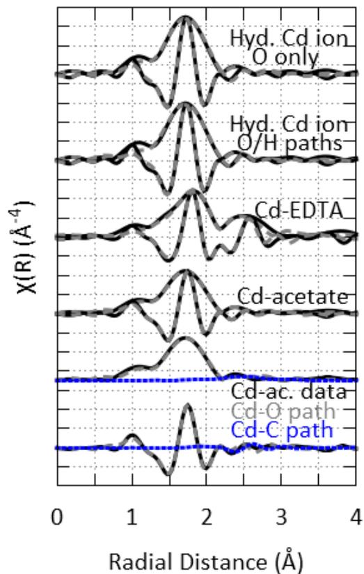
Fig. S.2: Fourier transformed (FT) spectra of Cd(II) aqueous standard compounds showing both the magnitude (all positive) and real part of the data (solid black line) and the best fit line (dashed gray line). The bottom shows example fitting paths of the Cd-O path (dashed gray line) and the Cd-C path (dotted blue line) for the Cd-acetate fit (black line) in both magnitude (top) and real part (bottom) of the FT spectra.
